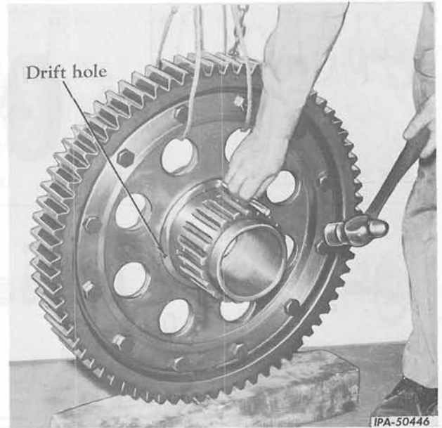
Illust. 15 - Removing the Inner Bearing.
